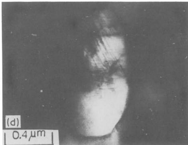
Figure 5 TEM micrographs illustrating the presence of twinning in all four \{111\} planes in a strontium-modified fibre. Al-14% Si-0.18% Sr. v = 330 \mu\text{m sec}^{-1} , G = 50^\circ \text{C cm}^{-1} (a), (d), (g), (l): Bright field micrographs of the same fibre segment with electron beam parallel to four different \langle 110 \rangle crystal orientations; (b), (e), (h), (m): Kikuchi line patterns at (a), (d), (g), (l); (c), (f), (j), (o): Key to Kikuchi patterns; (i), (n): Diffraction patterns taken from the fibre segment for its [011] and [0\bar{1}\bar{1}] orientations; (k), (p): Keys to diffraction patterns.
