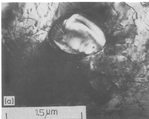
Figure 8 TEM micrographs showing \{111\} twinning in impurity modified silicon fibre. Al–14% Si–0.18%Sr, v = 89 \mu\text{m sec}^{-1} , G = 50^\circ \text{C cm}^{-1} . (a) Transverse section, bright field micrograph, exhibiting two intersecting sets of cozoal twin traces belonging to \{111\} twin planes; (b) Dark field micrograph selecting one of the two twin orientations in (a).
